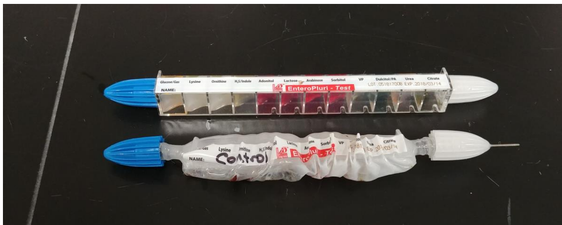
Figure 7. Un-autoclaved enterotube (top) and autoclaved enterotube (bottom). The enterotube inoculating needle protrudes from the media holder after autoclaving resulting in a sharps hazard.
